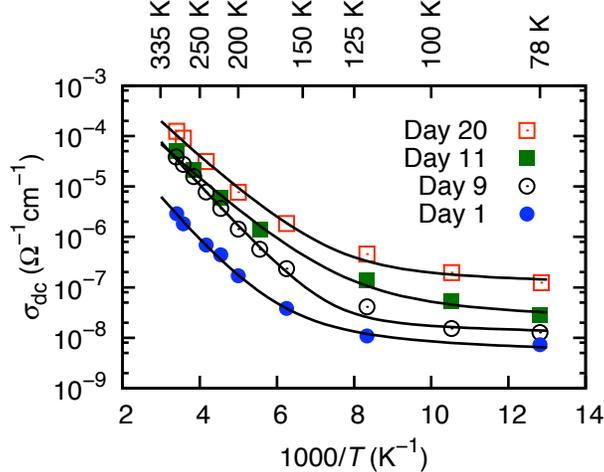
Figure 1. Temperature dependence of the DC conductivity of the SnO<sub>2</sub> sample. Solid lines illustrate the FITC model fitting. The corresponding fitting parameters are listed in Table 1.
