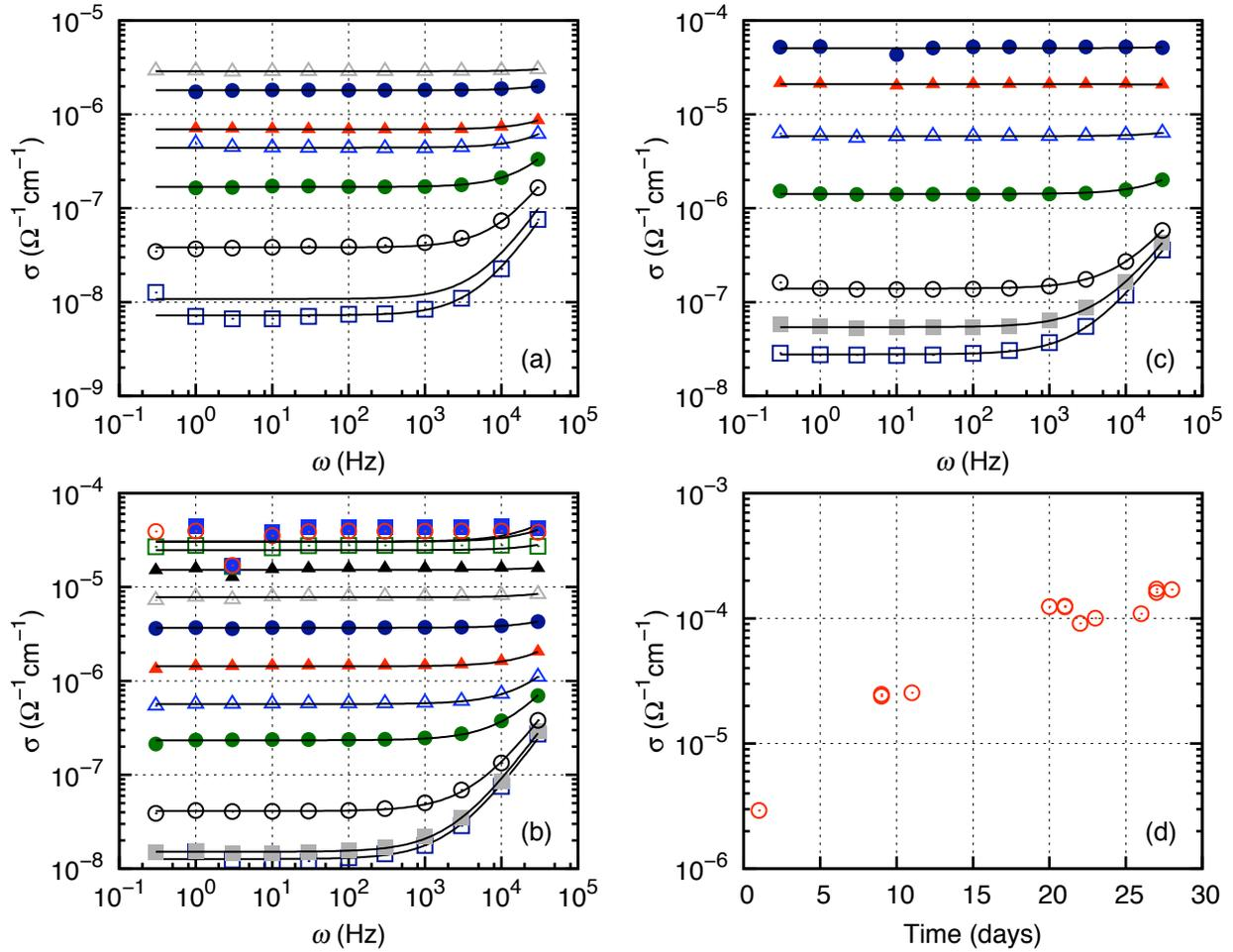
Figure 2. (a), (b), and (c): Frequency-dependent AC conductivity of the  $\text{SnO}_2$  sample as a function of temperature measured on days 1, 9, and 11. Solid lines illustrate power law fits to equations (1) and (2). (d): Drift of the DC conductivity over the course of 28 days of measurement.
