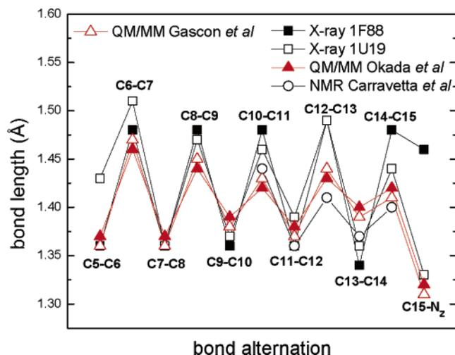
**FIGURE 7.** Bond-length alternation along the polyene chain of the 11-cis retinyl chromophore in rhodopsin, including the X-ray crystal structures 1F88, 1HZX, 1L9H, and 1U19, the QM/MM-MD (SCC-DFTB:CHARMM) structure,<sup>5</sup> a recent NMR structure,<sup>32</sup> and the QM/MM ONIOM-EE (B3LYP:AMBER) model.<sup>1</sup>
