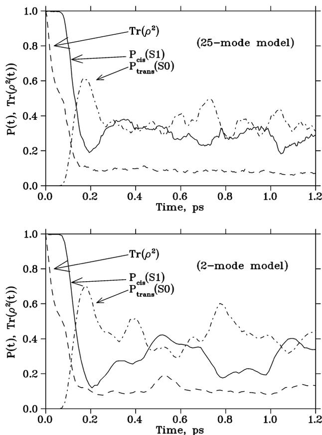
**Figure 4.** Comparison of the evolution of the  $\text{Tr}[\rho^2]$  (dashes) with the evolution of the time-dependent reactant cis- $S_1$  (solid lines) and trans- $S_0$  (broken dashes) populations during the first 1.2 ps of dynamics after photoexcitation of the system.
